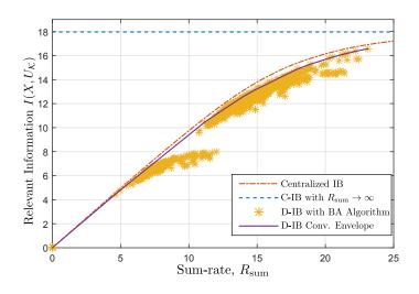
Performance of distributed-IB is close to that of centralized IB
